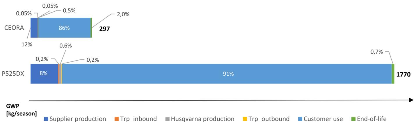
Figure 6 Contributions to GWP during usage in the EU. Values given at the far right of each column represents the GWP per cutting season.
