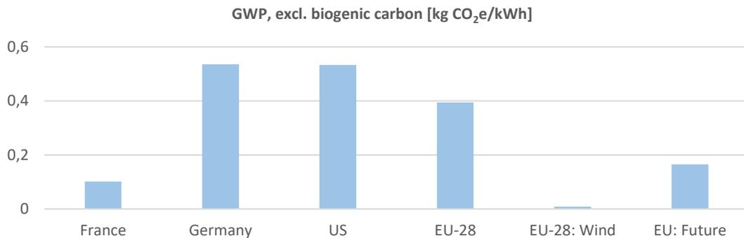
Figure 2 Global Warming Potential related to the electricity mixes used in the assessment.
