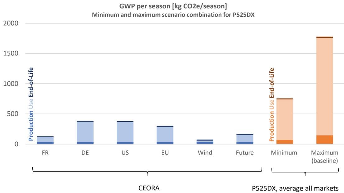
Figure 12 Sensitivity analysis with combined scenarios for P525DX compared to baseline
