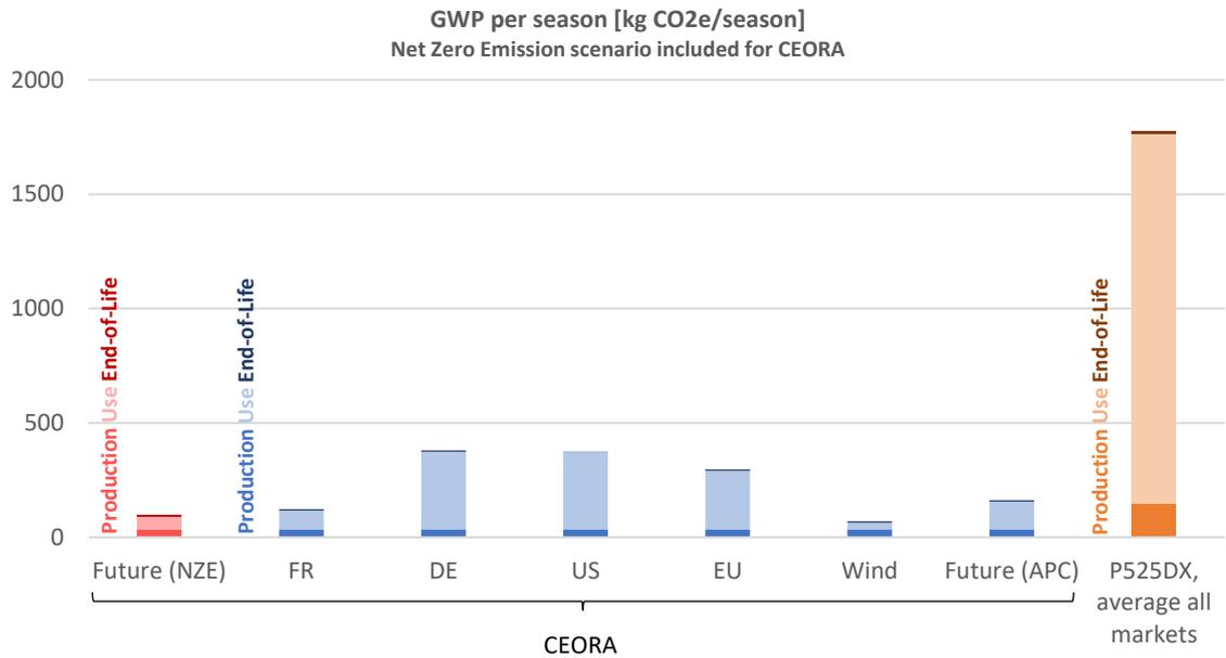
Figure 9 Sensitivity analysis with NZE scenario as energy source in the use phase for CEORA
