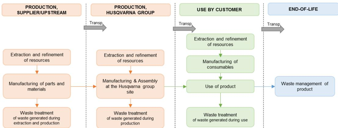
Figure 1 Simplified process tree. Orange marks the Production phase, green the Use phase, and blue the End-of-Life phase
