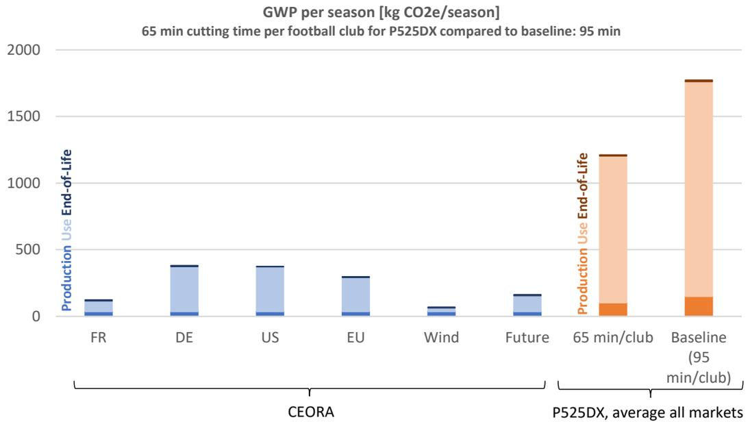
Figure 11 Sensitivity analysis with reduced rider cutting time compared to baseline results
