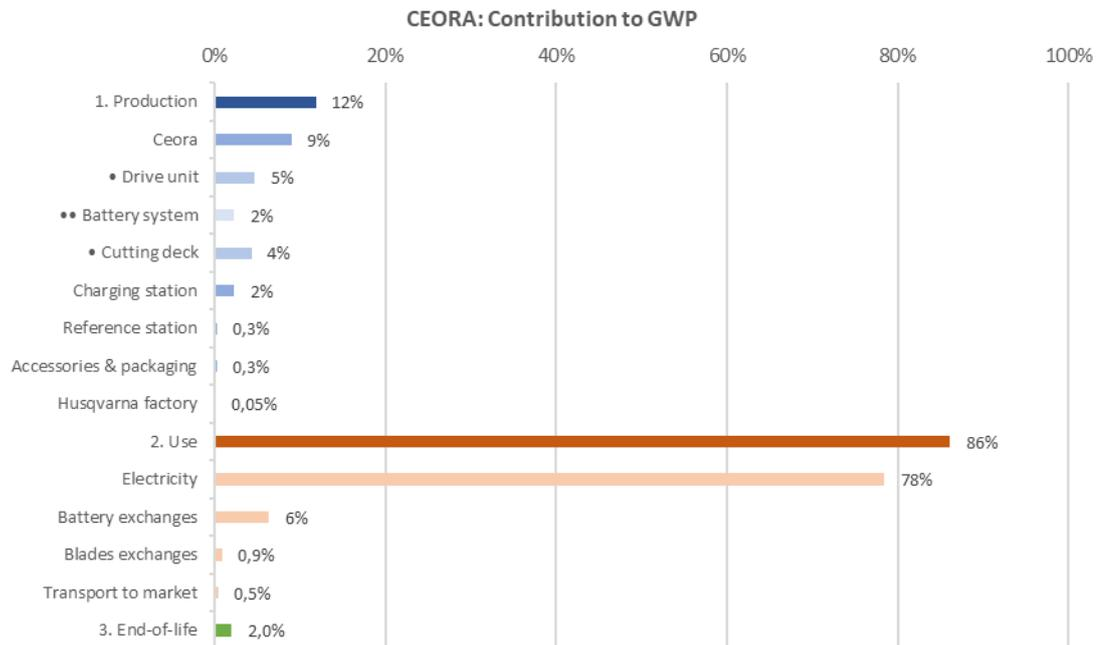
Figure 4 CEORA contribution distribution to Global Warming Potential during typical usage in the EU market. The blue bars present the Production phase, the orange the Use phase and the green the End-of-Life phase. The bars with the life cycle stages names and the numbers 1-3 present the total for this phase, while the remaining present their shares. The symbol "•" indicates that this part/process is underlying the closest part/process above.
