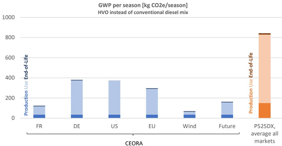
Figure 7 Sensitivity analysis for using 100% HVO in P525DX instead of conventional diesel
