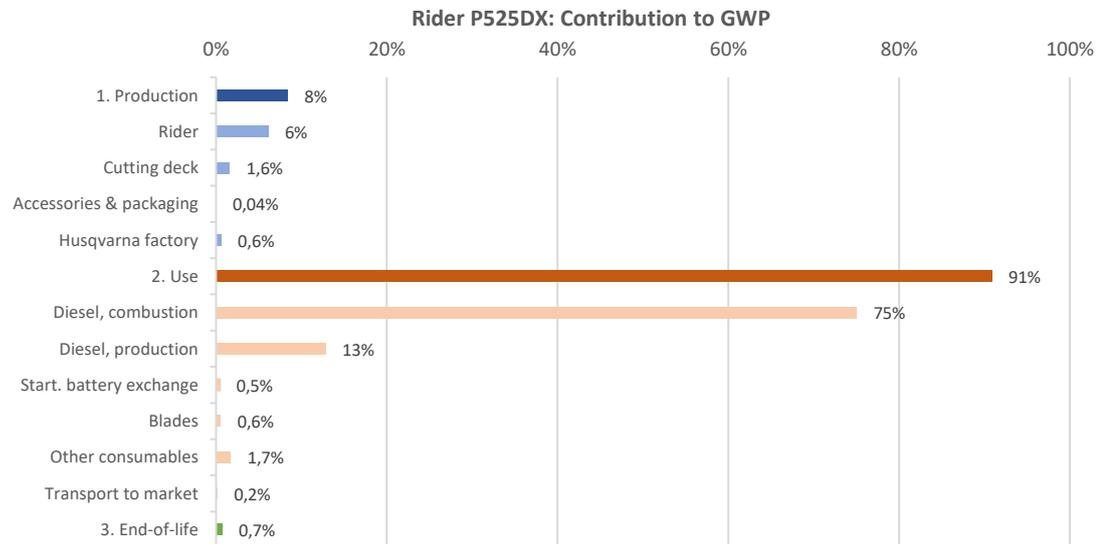
Figure 3 Rider P525DX contribution distribution to Global Warming Potential during its lifetime. The blue bars present the Production phase, the orange the Use phase and the green the End-of-Life phase. The bars with the life cycle stages names and the numbers 1-3 present the total for this phase, while the remaining present their shares.
